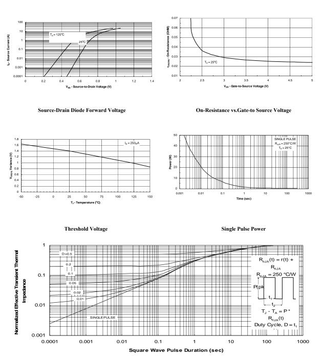
Typical Electrical Characteristics (N-Channel)
